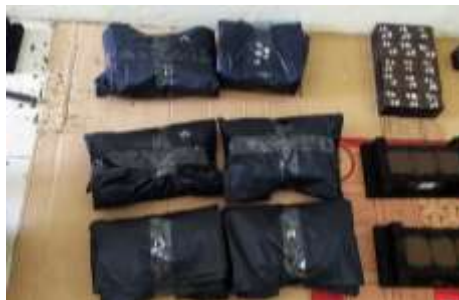
Gambar 7 Proses Perawatan/Curing Benda Uji Mortar Geopolimer
