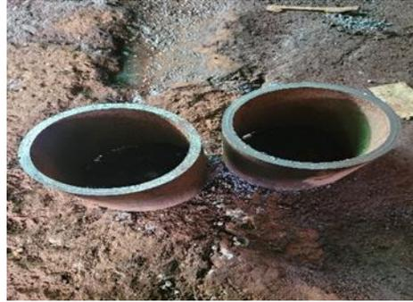
Gambar 4 Pipa Seamless Sch 40.
